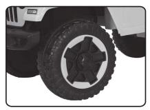
3. Instale as calotas e as parafuse
